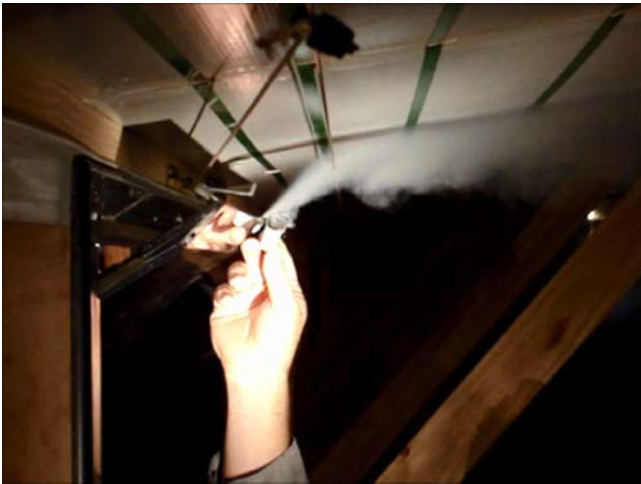
Figure 4. Air entering a house moving parallel to the ceiling.
