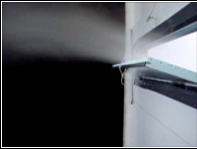
Figure 6. Wider inlet openings tend to result in incoming air moving more parallel the ceiling.
