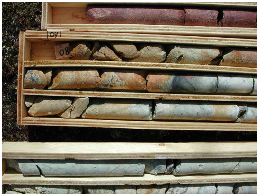
Illustration 1: Drill core from the Kiggavik deposit, Nunavut, illustrating the gradation from hematite alteration (red) through bleach clay alteration (biece) to deposition of uraninite (a uranium mineral, black).
