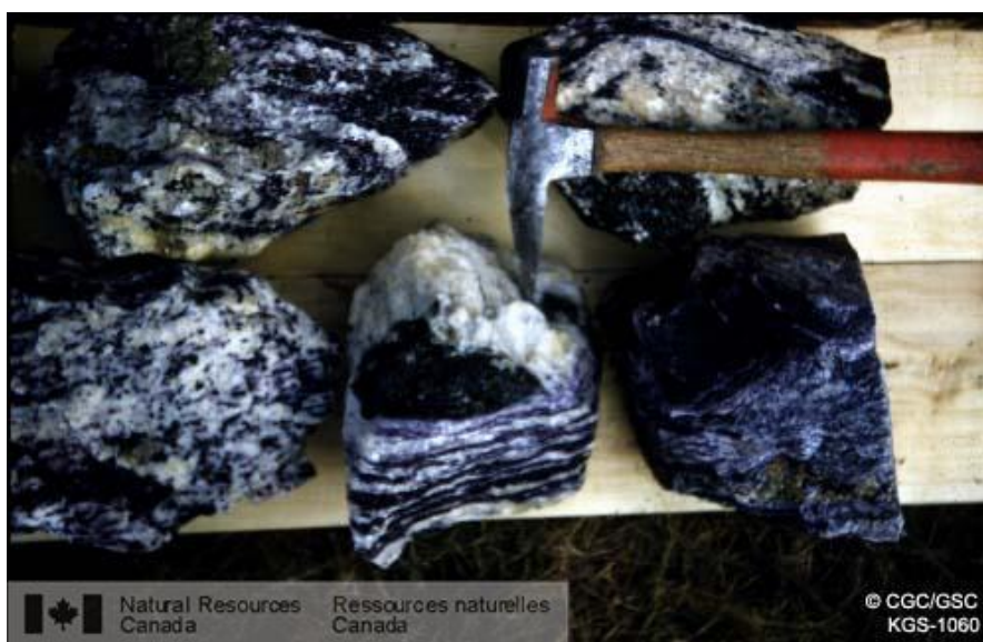
Illustration 2: Calcite (white)-fluorite (purple)-apatite (yellowish)-uraninite (black) ore from the Cardiff Uranium Mine at Wilberforce, Ontario. (NRCan Photo Library, Ottawa, Photo Number KGS-1060).
