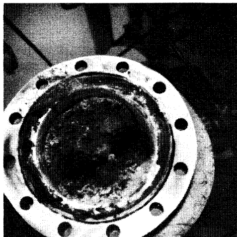
FIG.10. Caking of bed material in the upper cone part of the reactor.
