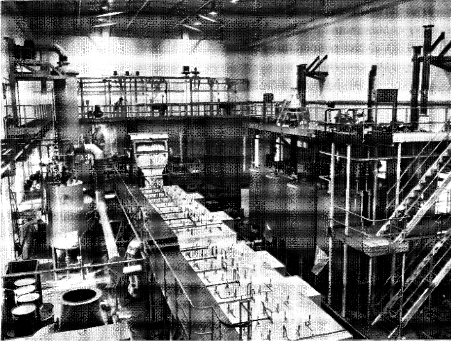
FIG.12. Overall view of pilot plant for converting ammonium diuranate into ammonium trioxide.
