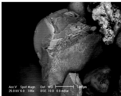
Fig. 5: Copper carbonate mineral (malachite), very bright spot (up-right), near kaolinitic grain
