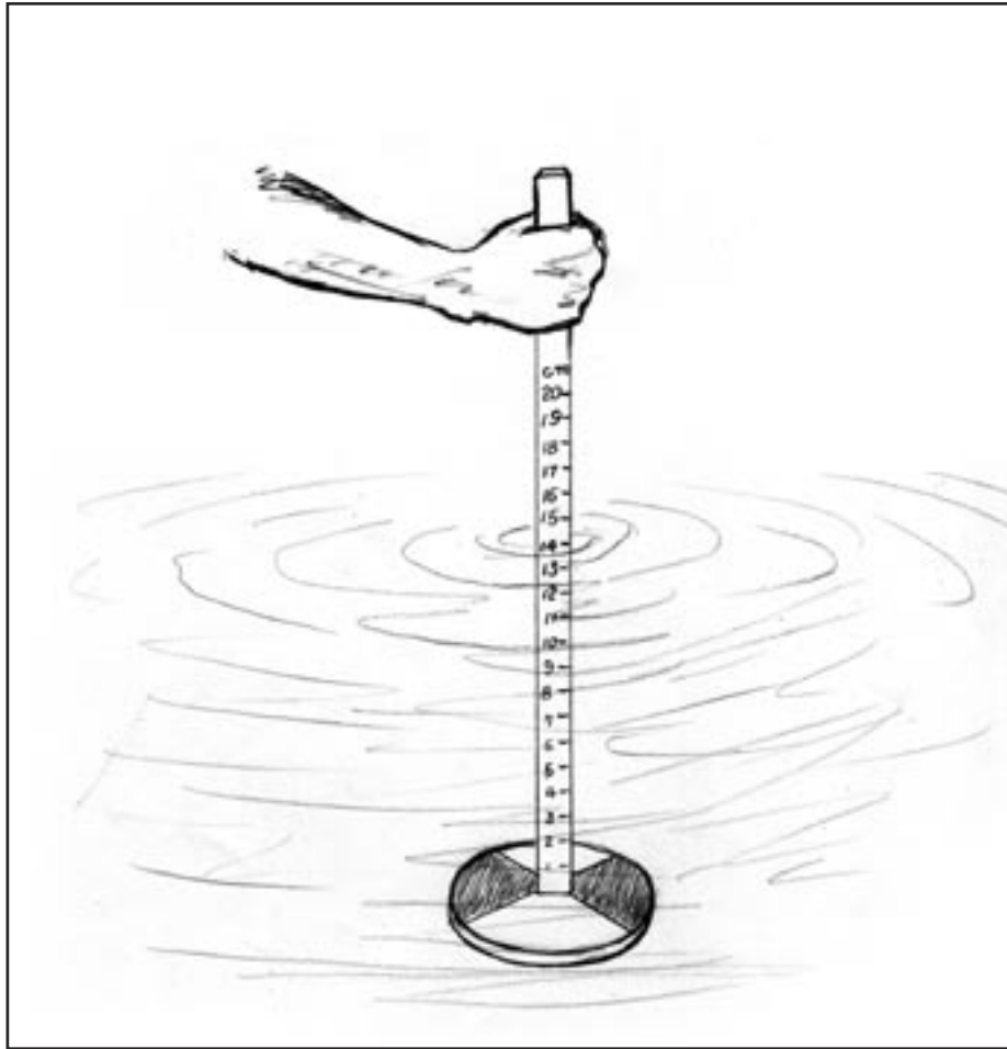
Fig. 16 A Secchi disc. The water depth at which the black-and-white disc just disappears from view underwater can be read off the centimetre scale drawn on the handle
