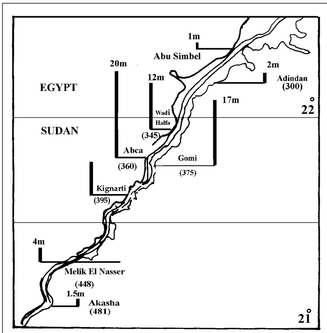
Fig. 14 Distribution of siltation in the Aswan High Dam Reservoir. Figures in parentheses indicate distance (km) from the High Dam (Latif 1984a).
