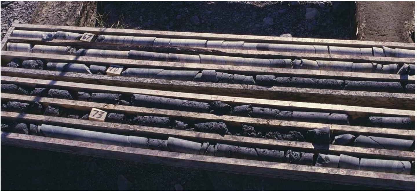
Fig. 7: Unconformity-related uranium ore in the Athabasca sandstone: Drill core from the Pod 2 area of the McArthur River deposit, Saskatchewan, Canada. DDH 301 consists over several meters of very-high-grade (> 50 % U) friable uraninite and argillic minerals. (Photo: Lehmann).
