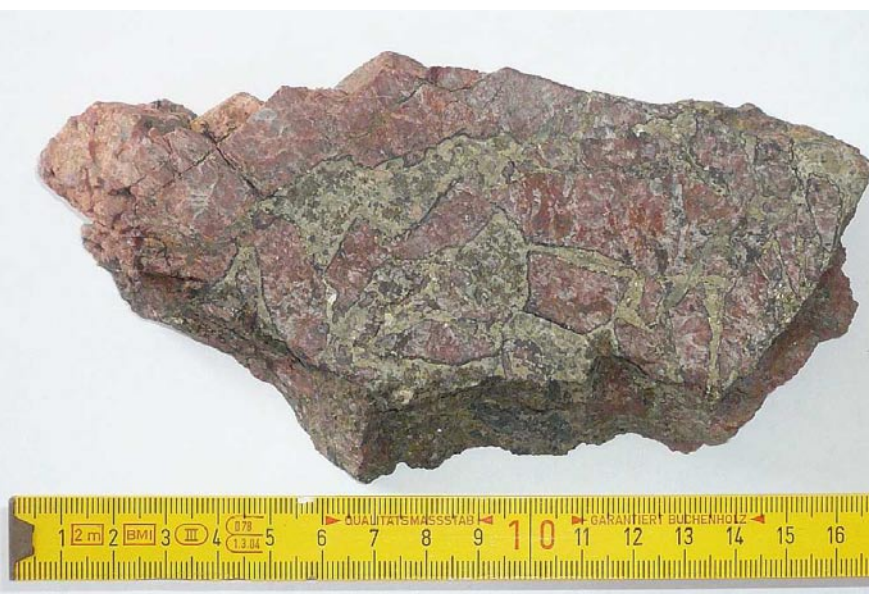
Fig. 4: Uranium ore from the Bertholène deposit (mined out) in the Massif Central, France. This granite breccia consists of hematitized granite fragments (red), cemented by thin uraninite rims (black), followed by pyrite (yellowish), and demonstrates the change in oxidation state of the system from oxidized (hematite) to reduced (pyrite). Uraninite is precipitated during this change in redox conditions. The ore occurs near the unconformity of weathered Hercynian granite of Carboniferous age and overlying Permian coal-bearing strata of Permian age. (Sample collection Lehmann).
