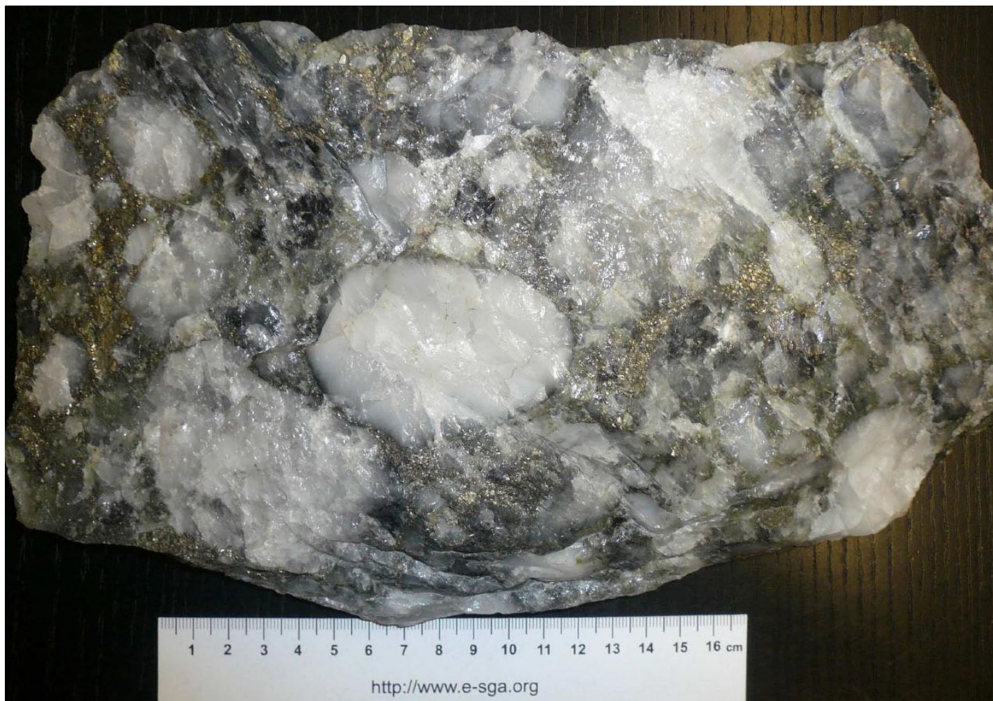
Fig. 12: Paleoplacer gold-uranium ore, Ventersdorp Contact Reef, Witwatersrand, South Africa. This typical sample shows milky-white quartz pebbles in a fine-grained matrix of chlorite and pyrite (yellowish). Uraninite and gold are visible under the microscope only. Average grade of the 3.1 Ga Witwatersrand paleoplacers is about 10 g/t Au + 210 g/t U, while the very similar Blind River/Elliott Lake paleoplacers in Canada have 900 g/t U, but no gold. (Sample collection Lehmann).
