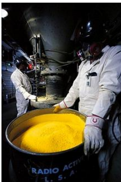
A uranium mine's end product: yellow cake, a uranium concentrate that is packed and shipped in containers. Picture from http://www.istockanalyst.com/finance/story/4943940/-100-uranium-on-the-horizon . Viewed 14 April 2011.
