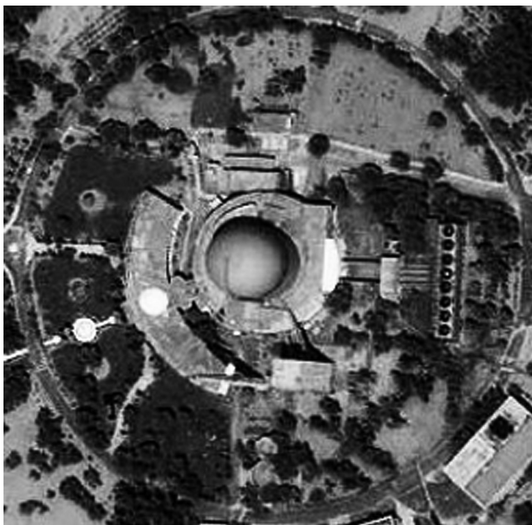
Figure 1: Khushab I reactor—the reactor building is at the center and the eight cooling towers are at the right (IKONOS satellite imagery courtesy of GeoEye).
