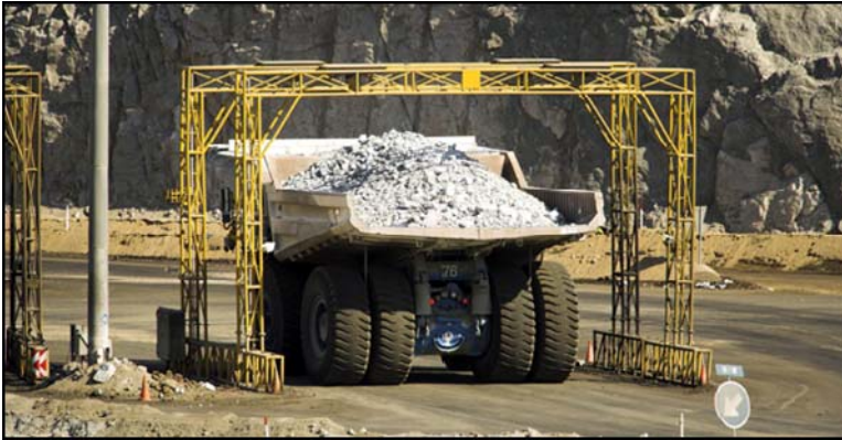
Plate 4.1: Rössing, with almost 35 years of production, is the most established uranium mine in Namibia. In this photo, an ore truck passes under a scanner to determine the ore grade (photo Geological Survey).
