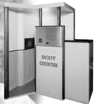
Whole body counter that measures internal contamination levels
