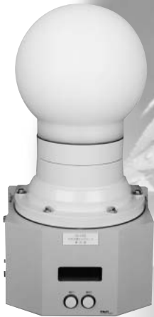
Detector that measures neutron dose rates
