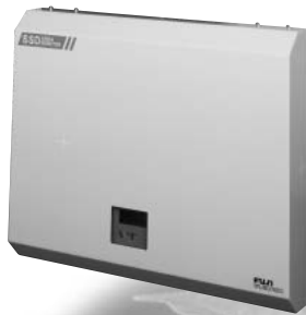
Detector that measures gamma-ray dose rates
