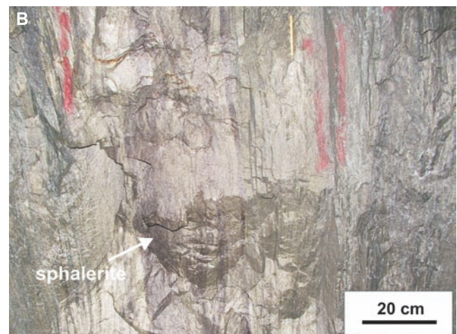
FIGURE 10. (A) Massive pyrite zone, lens 20 North, LaRonde Penna. (B) Massive pyrite with layers of sphalerite, lens 20 South, grading 34 g/t Au and 8% Zn over 10 metres, LaRonde Penna.
