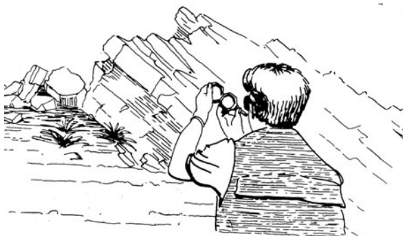
Fig. E.2 Sighting with a geological compass along the strike of an outcrop to obtain the average dip of beds exposed on vertical surfaces. Caution, the line of sight must be parallel to strike
