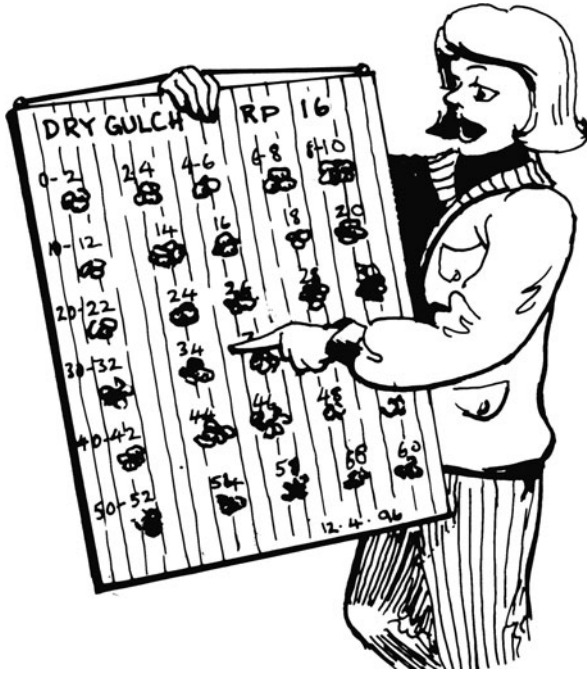
Fig. 6.4 A permanent display of washed cuttings. Cuttings from a typical hole or section are glued to suitably labelled board. The board can then be used as a reference for future logging, to maintain consistency of description between geologists, or for presentations
