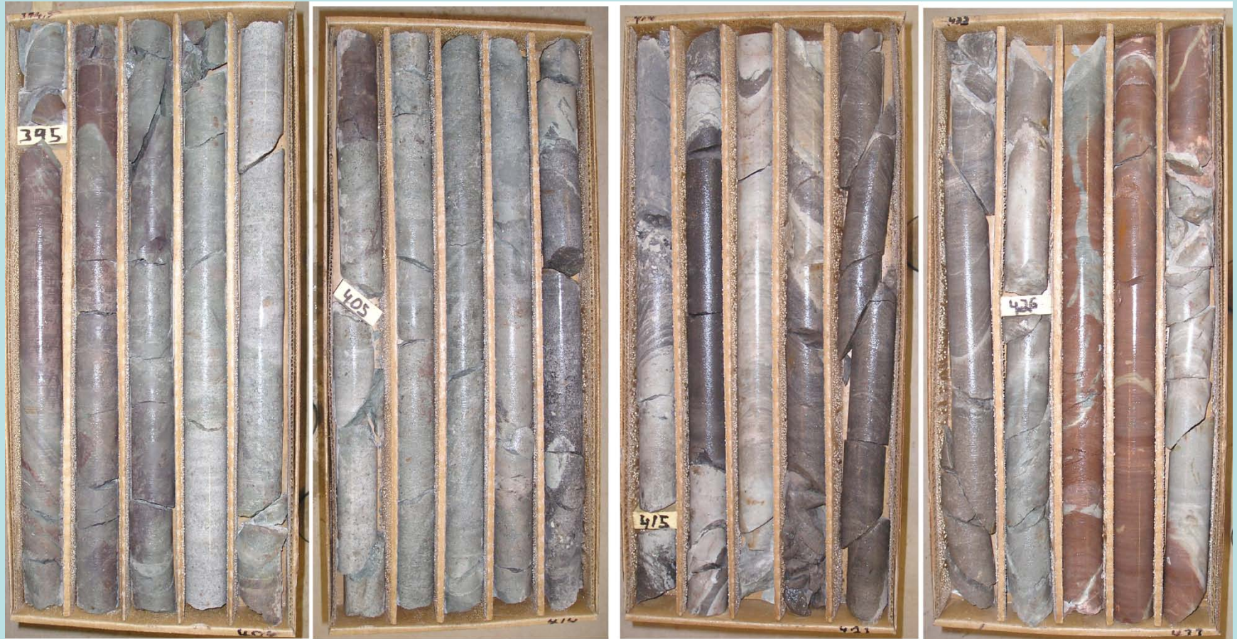
LV 4C3 395 to 433 - bitumen impregnated sandstone and conglomerate Basal Chinle Fm. (contact with Cutler at 425 ft)
